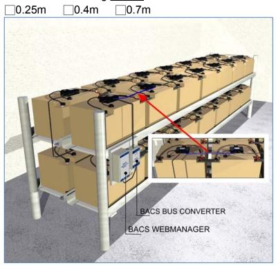
Enter the length in cm that a bus cable is required to be in order to connect two **BACS** modules on batteries standing <u>behind</u> each other.
